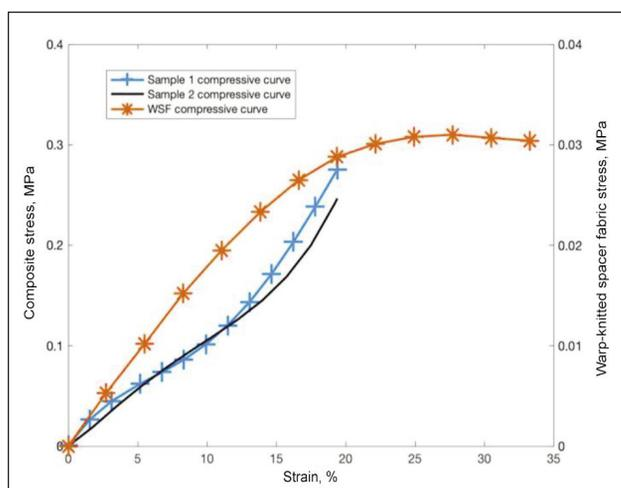
Fig. 2. The stress-strain curve of the compressive experiment
