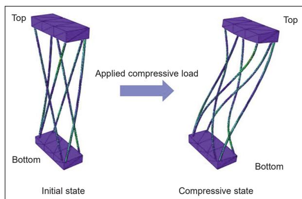
Fig. 3. The schematic of compression deformation of WSF
